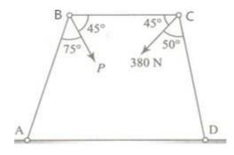
2. Find the axial forces in each member of the loaded frame ADBEC as shown in the below figure.
